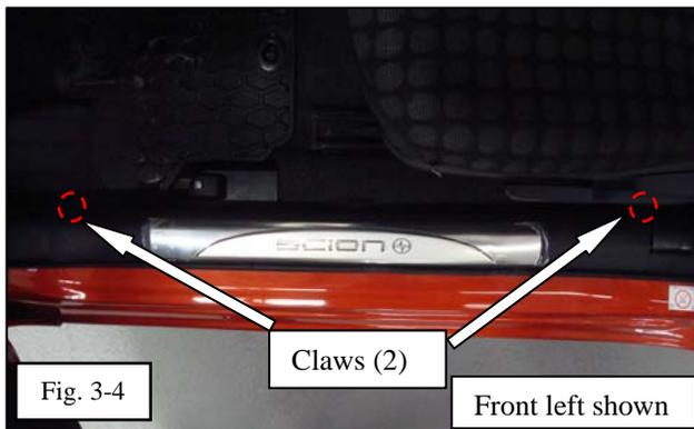
**3. Install left (driver side) and right (passenger side) door sill enhancements.**
